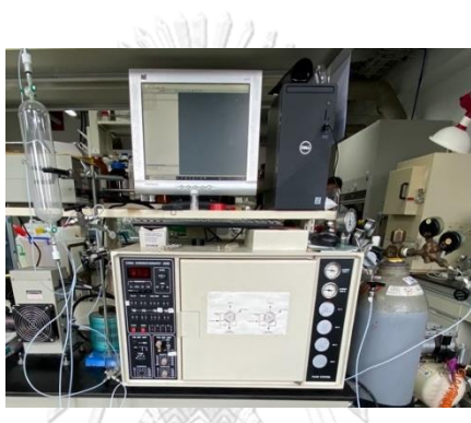
Figure 3-3 Gas Chromatography (China Chromatography 2000) and Thermal Conductivity Detector
