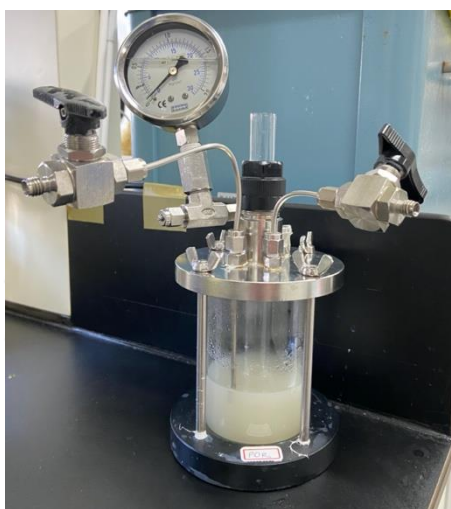
Figure 3-1 300 ml Pyrex glass reactor
