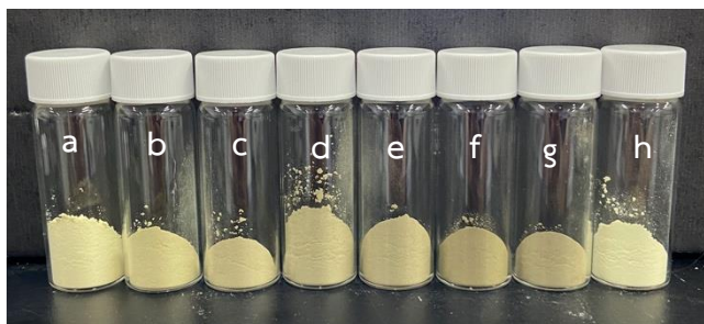
Figure 4-9 Colors of (a) gCNS, (b) 1CoB-gCNS, (c) 3CoB-gCNS, (d) 5CoB-gCNS, (e) 7CoB-gCNS, (f) 9CoB-gCNS, (g) 11CoB-gCNS, and (h) 7NiB-gCNS
