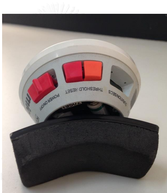
Figure 3.5 Knee extension force was measured by the microFET 2 hand-held dynamometer.
