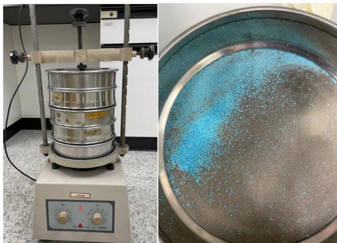
Figure 3-5 PVC microplastics preparation
