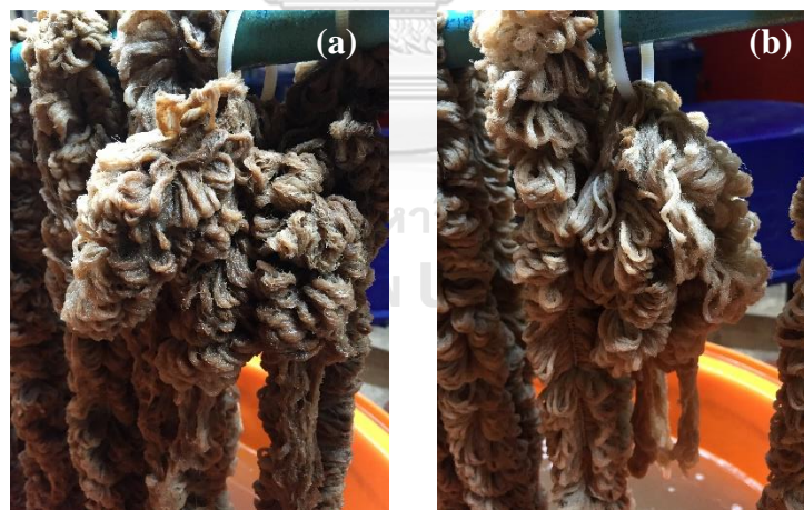
Figure 48. (a) Before and (b) after cleaning of fibrous Biocord™ biofilter during long-term operation of marine RAS.
