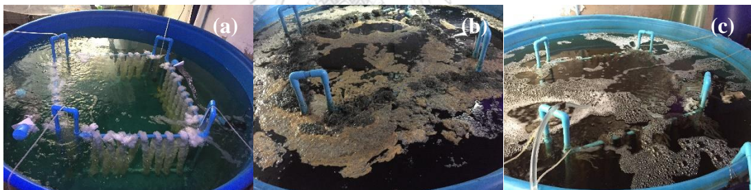
Figure 36. Experimental marine RAS for long-term operation of (a) biofilter acclimation with aerobic shrimp cultivation, (b) denitrification (anoxic, no shrimps) and (c) re-oxygenation, without water exchange.
