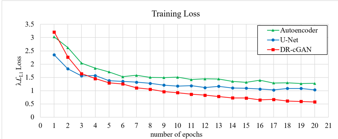
Fig. 2.22 Training loss comparison between Autoencoder, U-Net, and DR-cGAN on the UCSD Ped1 dataset.
