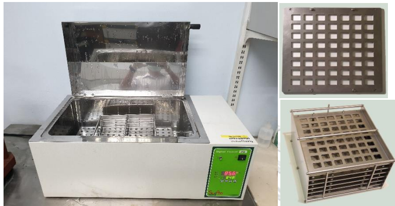
Figure 4.5 The water bath (Right) and the etch and scanning frame (Left)
