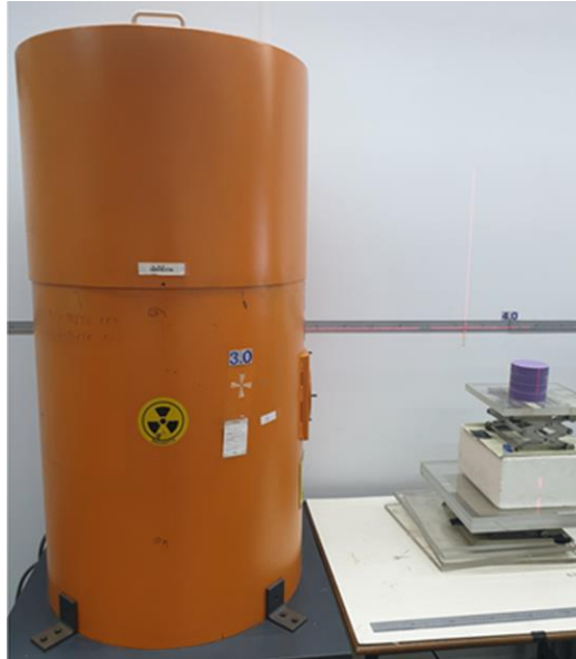
Figure 4.11 The calibration of CUMOD at 100 cm from the ^{241}\text{AmBe} calibrator source
