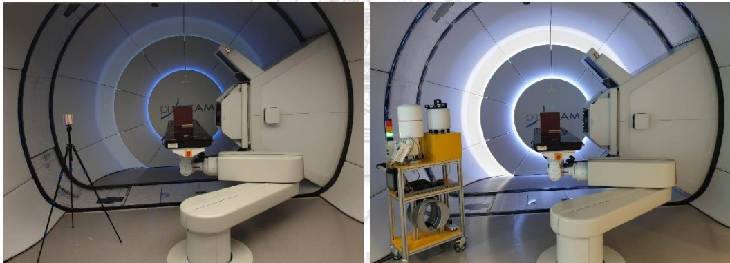
Figure 4.15 The measurement of H^*(10) of CUMOD and WENDI-II at proton therapy for high energy neutron response function validation.
