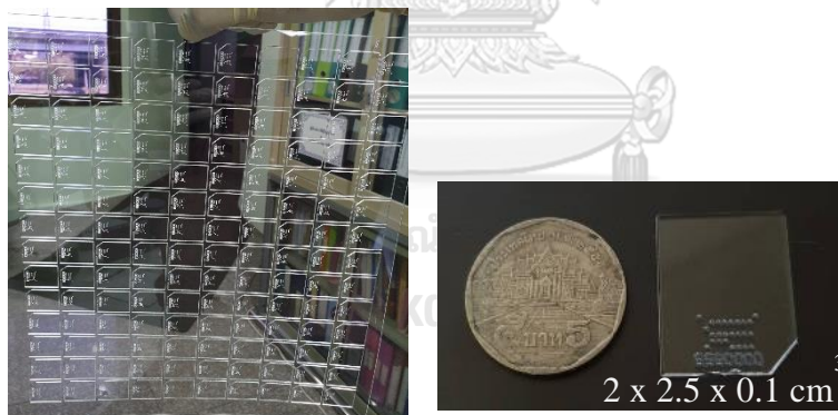
Figure 4.4 The whole plate and after cutting of CR-39
