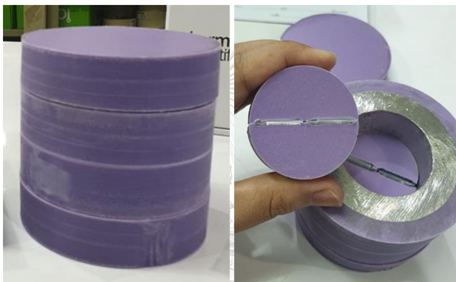
Figure 5.1 The Chulalongkorn University Neutron Moderator (CUMOD)
