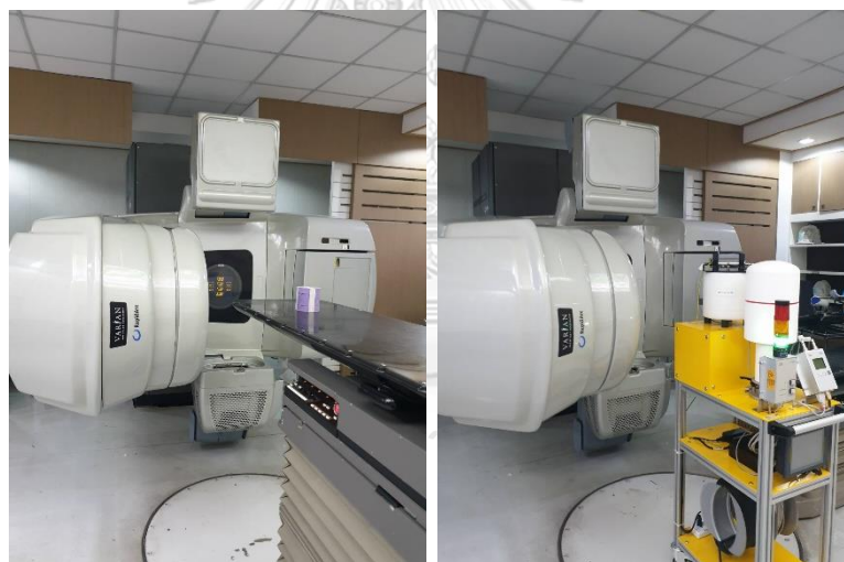
Figure 4.13 The measurement of H^*(10) of CUMOD and WENDI-II at Varian clinac 23EX for fast neutron response function validation.
