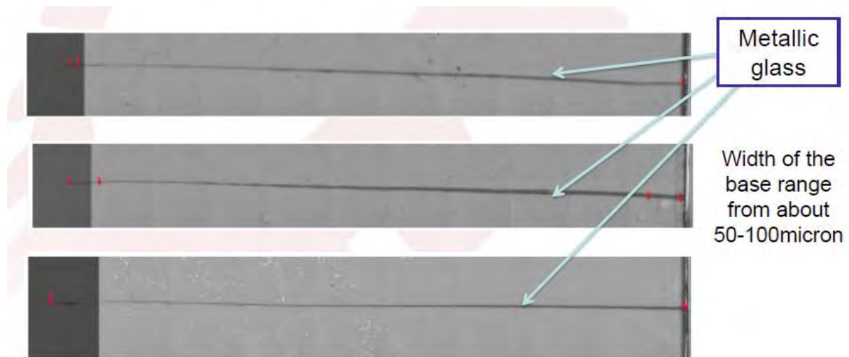
Figure 6 Pictures of metallic glass micropattern from inverted fluorescence microscope. Width of metallic glass micropattern were 50 – 100 \mu m
