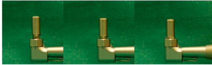
Figure 10 A guide tube directly screwed to the head of the surgical handpiece
