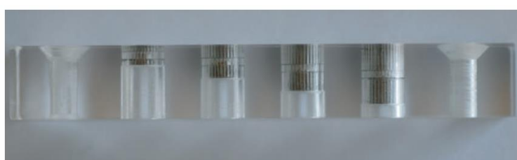
Figure 7 Surgical guide (from left to right) with different sleeve heights of 3, 5, 7 and 9 mm respectively.
