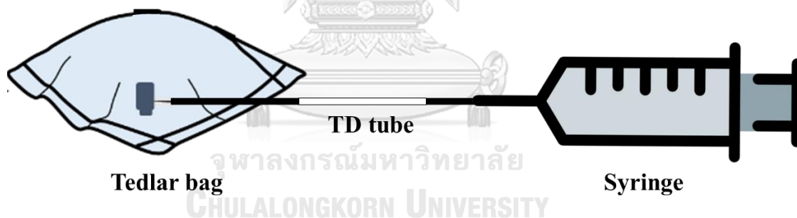
Figure 12. The method for sampling the standard gas from the Tedlar bag into the TD tube
