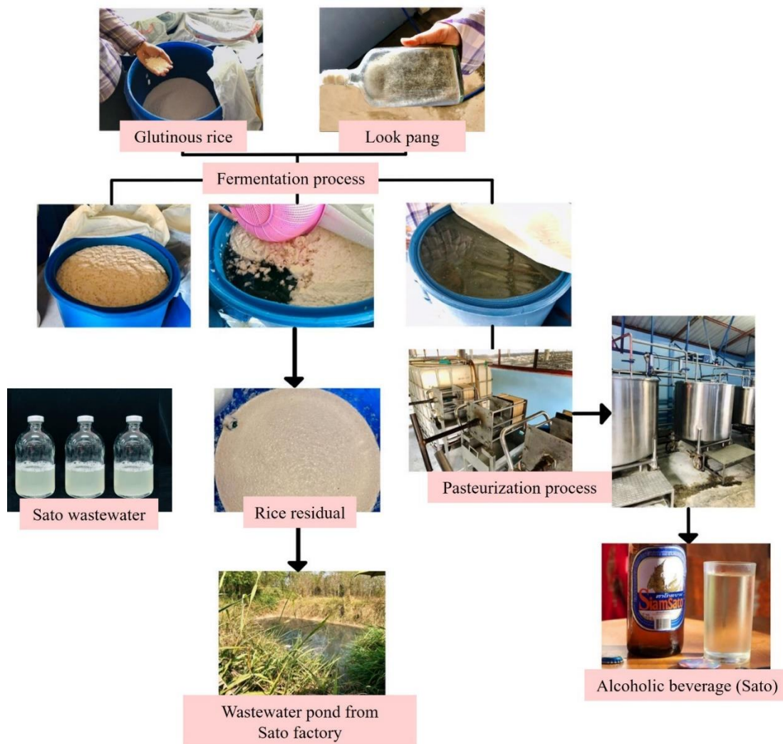
Figure 8 The Sato manufacturing process and its byproducts, including wastewater
