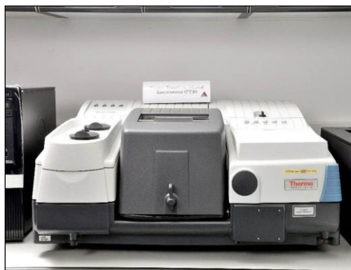
Figure 1.4 Thermo-Nicolet 6700 Fourier-Transform Infrared (FTIR) Spectrometer based at the Gem and Jewelry Institute of Thailand (Public Organization).
