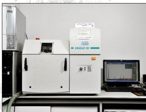
Figure 1.7 Eagle III system, Energy-dispersive X-ray Fluorescence (ED-XRF) spectroscope, based at the Gem and Jewelry Institute of Thailand (Public Organization).
