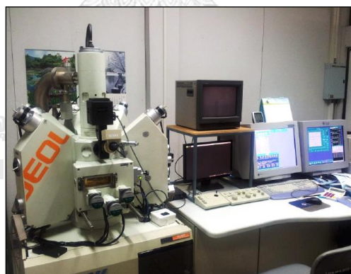
Figure 1.8 Electron Probe Micro-Analyzer (EPMA), Model JXA-8100, based at Department of Geology, Faculty of Sciences, Chulalongkorn University
