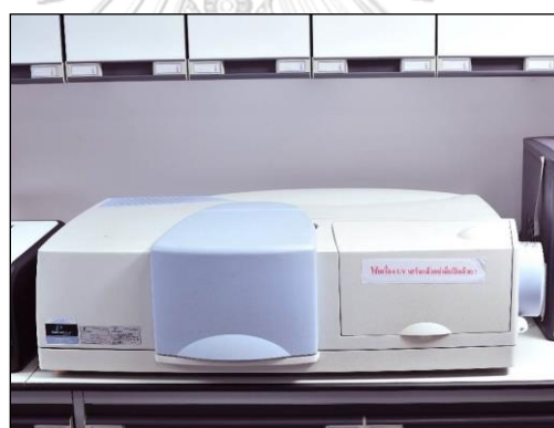
Figure 1.5 PerkinElmer Lambda 950 spectrophotometer based at the Gem and Jewelry Institute of Thailand (Public Organization).
