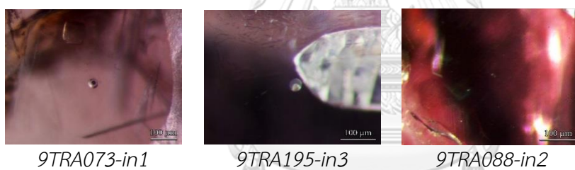
Figure B-6 Two-phase inclusions (sample 9TRA073 and 9TRA195) and anatase (sample 9TRA088) inclusions in Bo Rai ruby
