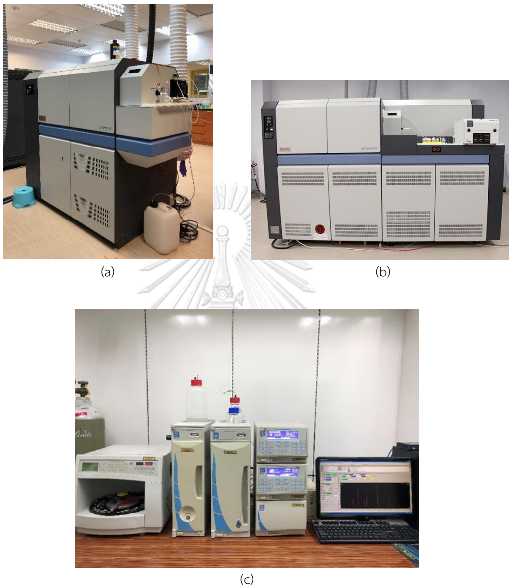
Figure 2.8 Analytical equipment (a) SF-ICP-MS (Element 2) Thermo Fisher Scientific for metal analysis, (b) Multicollector ICP-MS (Neptune Plus) Thermo Fisher Scientific for Pb-isotope analysis, and (c) Ion Chromatography (IC, ICS-2500, DIONEX) for water soluble ion analysis
