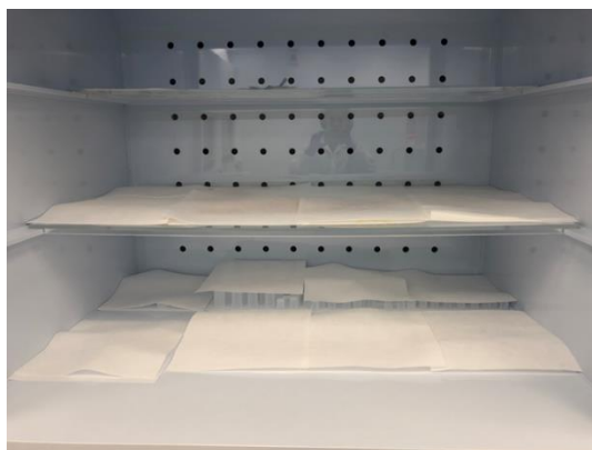
Figure 2.4 Drying precleaned PTFE filters in a laminar flow cabinet
