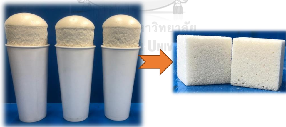
Figure 3.2 PIR foams prepared by cup test method and cut into the cubic shape
