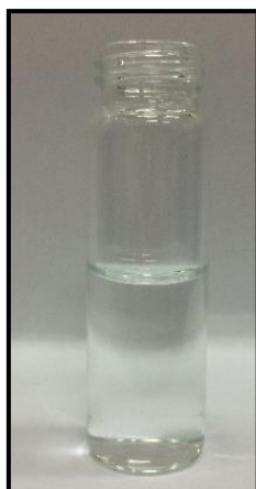
Figure 4.1 Zinc-ammonia complex Zn(Amm) aqueous solution
