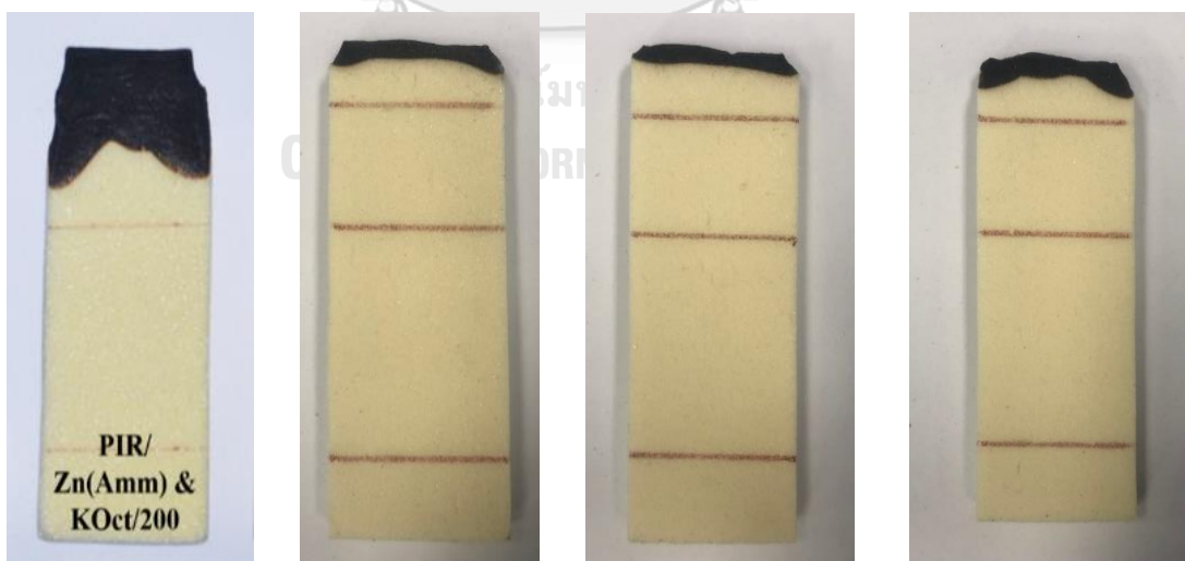
Figure 4.20 Appearance of PIR foams after burning test; (a) PIR foam is reference foam (b), (c) and (d) are PIR foams modified with glutinous rice flour, rice flour and mung bean starch respectively
