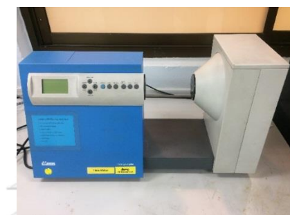
Figure 3.5 BYK-Gardner haze gard plus instrument (BYK-Gardner, Germany).
