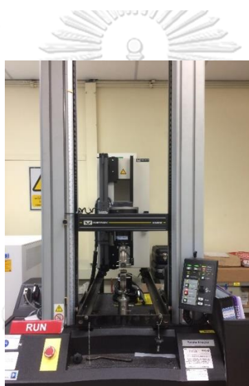
Figure 3.3 Film sample (a) Tensile strength test and (b) Tear strength test.
