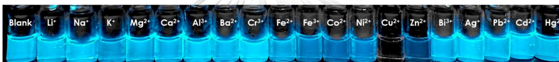
Figure 3.27 Photographed images of JS (10 \mu\text{M} ) towards various metal ions (100 \mu\text{M} ) in (a) DMSO and (b) 1:1 (v/v) DMSO and 50 mM HEPES buffer pH 8.0.
