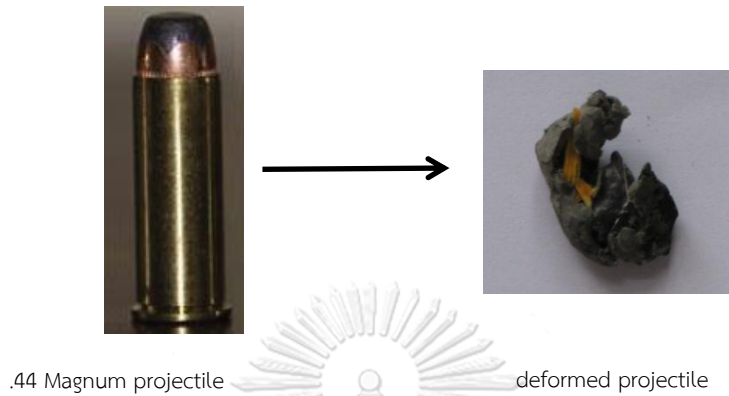
Figure 17: Deformation of .projectile after penetrated E-glass fiber reinforced PBA composite [78]
