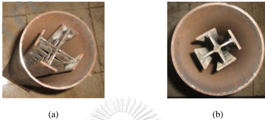
Figure 2.1 Steel reinforced-concrete filled with (a) castellated cruciform steel section; and (b) traditional cruciform steel section (Farajpourbonab et al., 2017).
