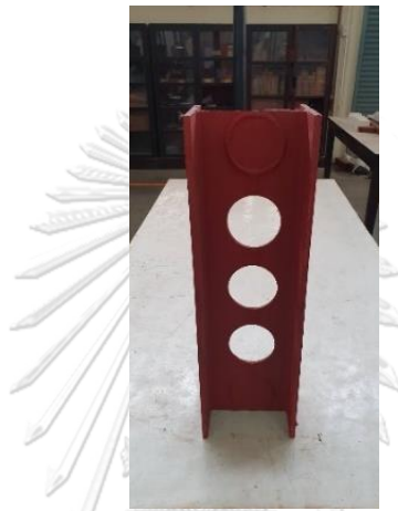
Figure 4.3 Cellular steel column (specimen ST-C1) after welding process.
