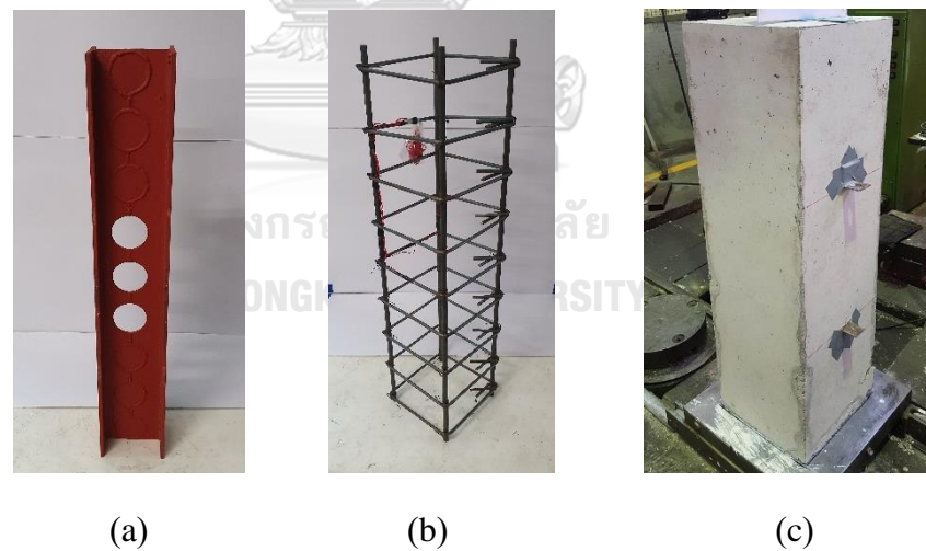
Figure 4.6 Components of CECS composite column (a) cellular steel; (b) steel reinforcements; and (c) composite column after concrete encasement.
