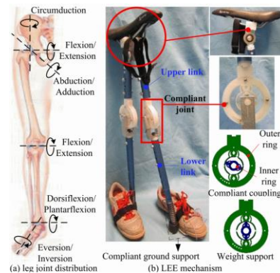
Fig 19 Design of the lower-extremity exoskeleton (LEE) [39].
