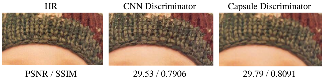
Figure 4.17: Visual comparison of our GAN model with capsule and CNN discriminator on a scale of \times 4 .
