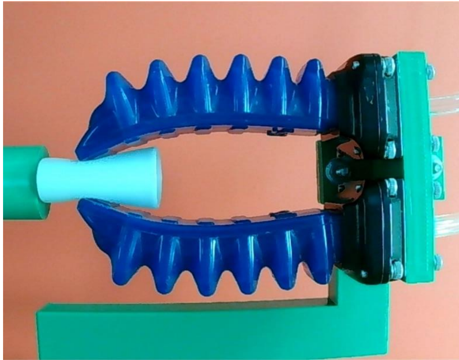
FIGURE 5. SPAs with continuously increasing angle of curvature along their length during SPG pincer grasping.
