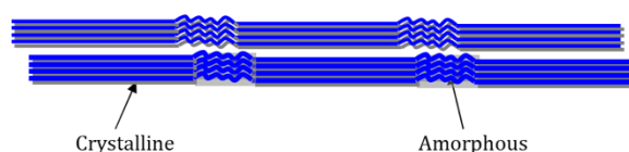
Figure 2.7 Crystalline and amorphous regions in cellulose microfibril [45]
