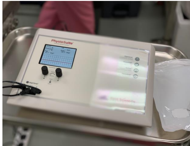
Figure 5 Temperature Monitoring and Homeothermic Control Module (RightTemp, Kent Scientific Torrington, CT, USA).
