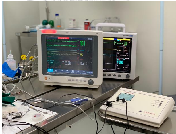
Figure 4 HR was measured by Electrocardiography (COMEN C80-V, Shenzhen Comen Medical Instruments Co.,LTD; Guangming, Shenzhen, CHINA). PR and SpO 2 were measured by pulse oxymetry (EDAN iM8 VET series, EDAN CHINA; Shekou, Nanshan Shenzhen, CHINA).
