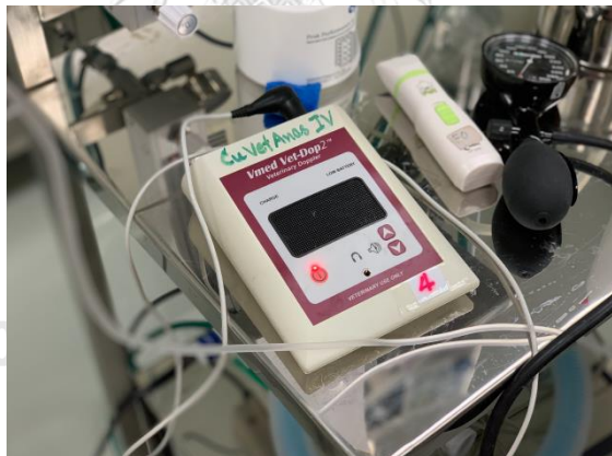
Figure 6 SBP was measured with a doppler blood pressure system (Vmed Vet-Dop2, Vmed Technology; Mill Creek, WA, USA).
