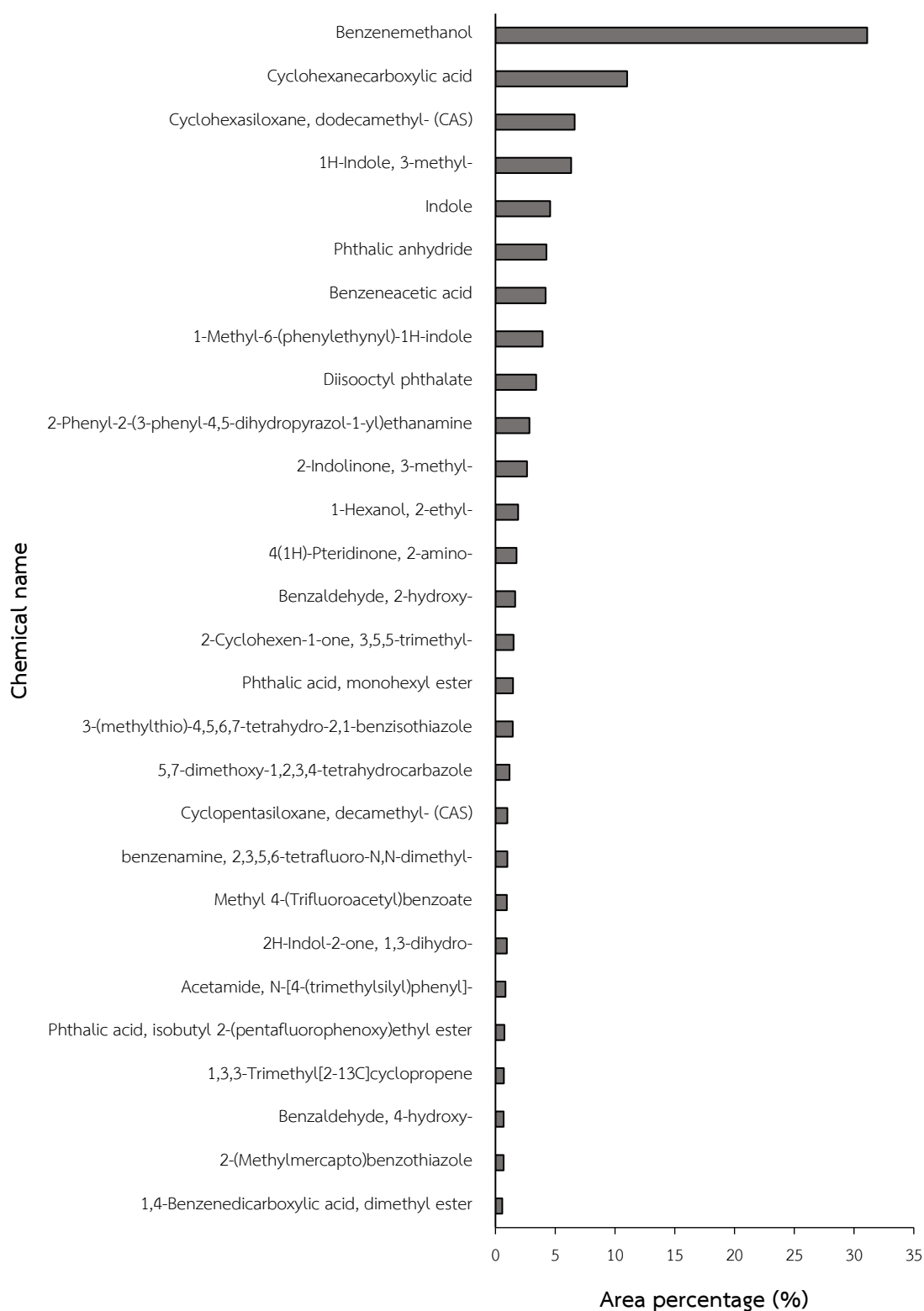
Figure 4.2 Organic compounds in influent wastewater obtained from wastewater receiving tank in factory S as evidenced by GC-MS.
