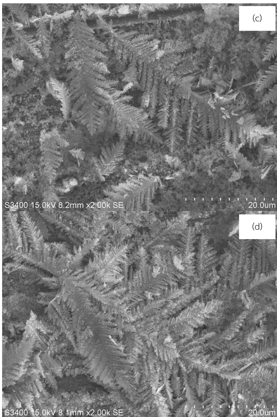
Figure 7 SEM images of (a) Zn foil, (b) Cu foil, (c) Zn/Cu-Na60, (d) Zn/Cu-Na200, (e) ZnCu/Cu-Na60, (f) ZnCu/Cu-Na200, (g) Zn/Cu-H60, (h) Zn/Cu-H200, (i) ZnCu/Cu-H60 and (j) ZnCu/Cu-H200
