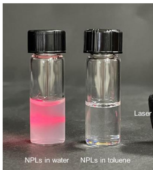
Figure S1. Light scattering of (left) the suspension of PSNSs in water and (right) the solution of PSNSs in toluene. NPLs particles with a particle size of approximately 800 nm were employed. The concentration of NPLs in toluene solvent (700 \mu\text{g/mL} ) was 10 times higher than that of NPLs in water media (70 \mu\text{g/mL} ).
