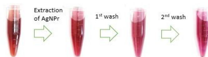
Figure 3.1 Digital images of the red citrate-capped AgNPrs throughout the centrifugation process.
