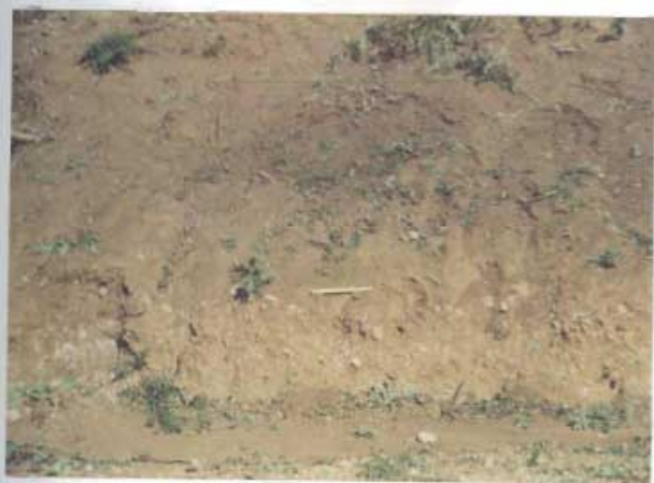
Figure 3.4 Thick basaltic soil covering gravel bed in the southern edge of the Sop Prap-Ko Kha basaltic area (grid reference 362854).
