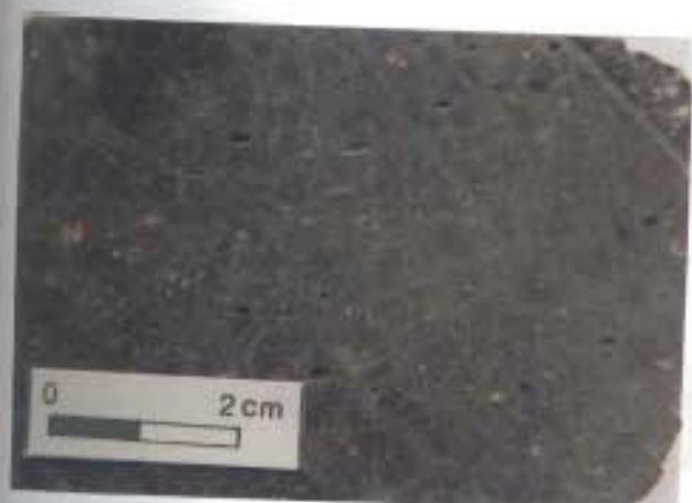
Figure 4.19 A specimen of the third flow of the Sop Prap-Ko Kha basalt showing vesicular, porphyritic, fine-grained, olivine basalt.
