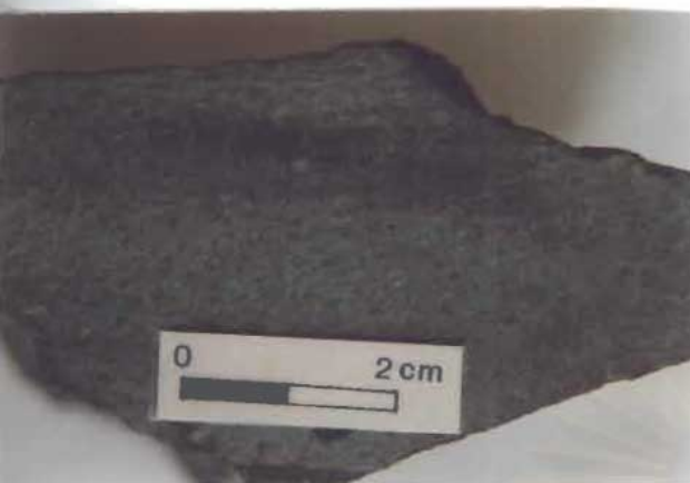
Figure 4.27 A specimen of the fifth flow of the Sop Prap-Ko Kha basalt showing fine-grained, porphyritic olivine basalt.
