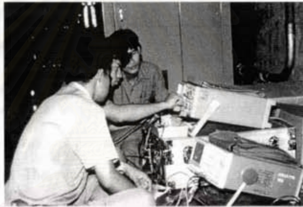
Fig. 3.3.14 Measuring unit and Coaxial cable trimming instruments
