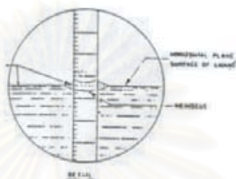
Figure A-2.1 Hydrometer scale reading for Transparent liquids
